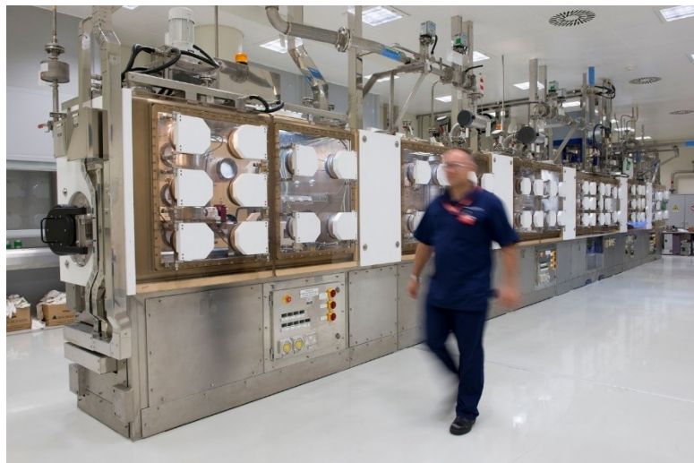
Figure 2: Glove boxes at the National Nuclear Laboratory (NNL) in the UK
