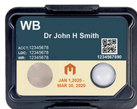
Figure 4 Image of a TLD (Thermoluminescent dosimeter)
