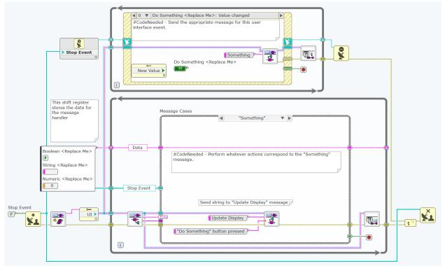
Typically, the event handler in the upper while-loop is responding to user actions and generating messages that is passed on the second while-loop at the bottom. This loop handles the hardware and acts upon the messages generated by the user event loop. Additional while-loops can be added to e.g. handle measurement timing and system safety. This is how the old RoboLabs were constructed.
